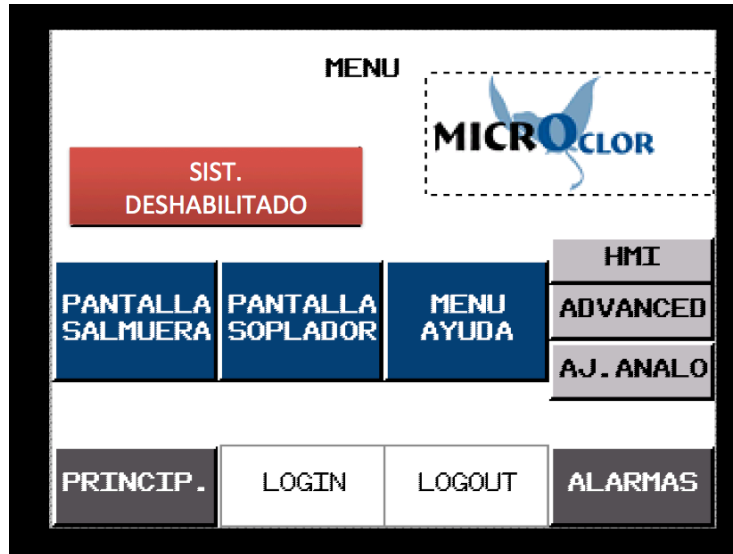
Figure 1: Showing the Disable System Button
