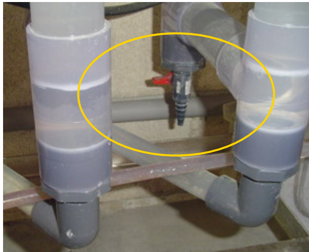
Figure 1 showing electrolytic cell drain stopcock at base of cells
